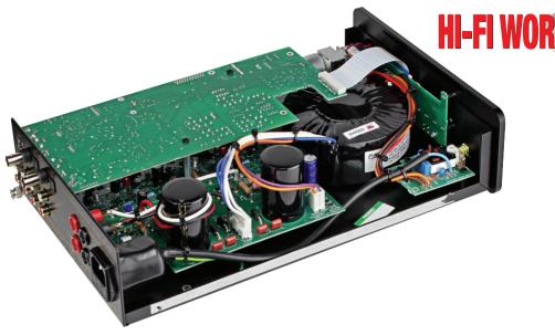
Exposure's neat but busy internal construction. The XM5's amplifier section is on the bottom, while the digital electronics occupy the top board. Both rely on the 200VA toroidal transformer that dominates the rear of the unit. In terms of running temperatures, the XM5 gave me no cause for concern.
