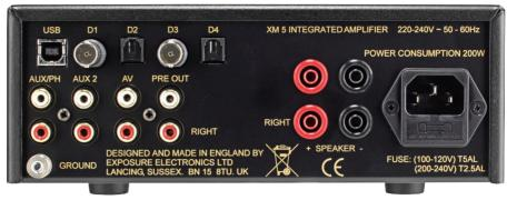
Plenty of connectivity, given the limited rear-panel real-estate. BNC sockets (D1, D3) accept S/PDIF digital for more accurate termination. Loudspeaker sockets accept 4mm plugs alone.
